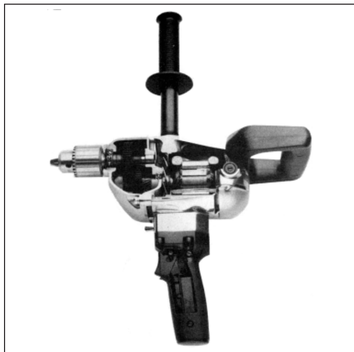
Figure 1. The gears in this Black & Decker heavy-duty drill account for much of its weight. The gears create high torque at the drill chuck by stepping down the rpm of the 9-amp motor.
