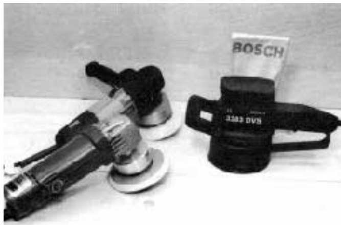
Random-orbit circular sanders let you sand across the grain without leaving sander marks. The three setups shown are a Marshco sanding head on a Makita grinder (far left in photo), a Porter-Cable model 7334 (top left), and a Bosch model 3283DVS (right).
