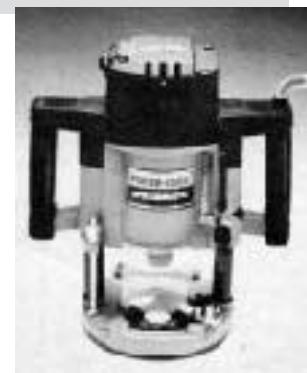
cooling, stiffer armature shafts to reduce vibration and bit run-out, and electronic speed controls. Of particular note is the model 7539 variable-speed plunge router. This production-size router has a 15-amp (3 1/4 hp) motor that runs between 10,000 and 21,000 rpm. These features make the tool comparable to the other variable-speed, plunge routers on the market (see Toolbox, 11/90).
