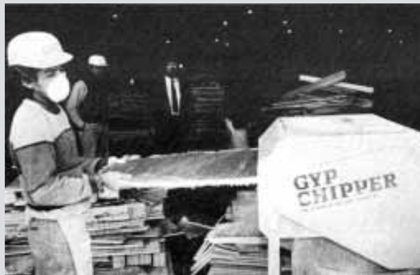
After running through the Gypchipper, ground-up drywall scraps are easily recycled into new gypsum products.
