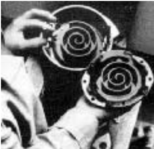
Figure 6. The new Copeland Compliant Scroll compressor is more efficient and reliable than conventional piston compressors. Most major heat pump manufacturers now sell models equipped with scroll compressors.
