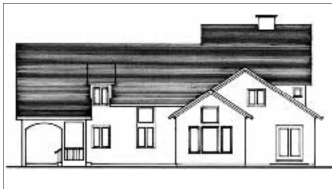
Figure 1. This facade from a recent project incorporates standard Andersen clad sash without any surrounding wood trim. It would have also been easy to work out the design using traditional windows with dividers. Here, modular windows are grouped to break up the house's long side. I always design windows from the inside out, and often (though not in this design) add exterior horizontal trim to organize the resulting hodgepodge.
