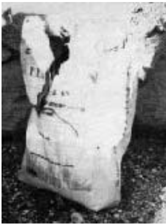
Freezing and exposure to the elements can undermine many tile materials — like this bag of mortar left in the weather overnight.
