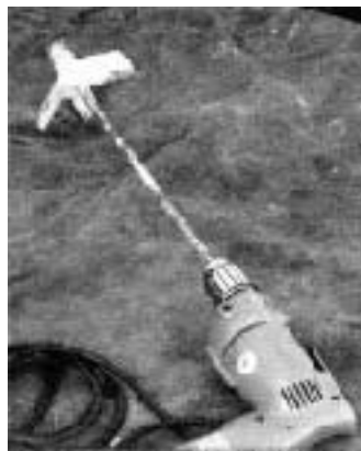
A mixing paddle for ceramic tile should have large, thick blades and run at about 300 rpm in a 1/2-inch drill. Smaller, faster blades will entrain air in the mix and weaken the grout.
