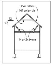
Aside from where this bracing method was used, I've never seen a kneewall over 16 inches in height that wasn't severely deformed, to the tune of about 3 inches over 40 feet.
