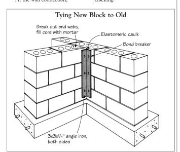
Secure block wall intersections with a vertical angle iron, as shown.
