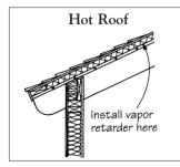
Moisture problems are likely in this roof assembly unless the interior vapor/air barrier is flawless. Also, because the roof is unventilated, there is a danger of heat buildup, which will reduce shingle life.
