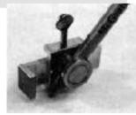
The McGrath Scribing Guide is a little-known English joiner's tool for scribing from woodwork and countertops to uneven walls and surfaces. This simple cast-aluminum jig replaces the gradeschool compass frequently used stateside. The jig holds a pencil at a fixed angle and has an L-shaped leg, which extends up to 13/s inches from the pencil-point. For longer
