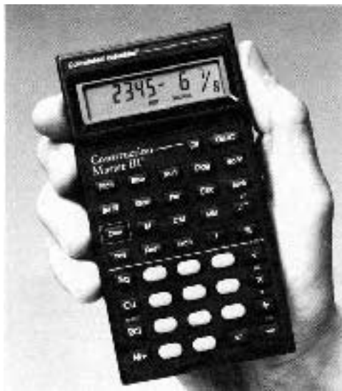
The new Construction Master III calculator simplifies on-site calculations, such as figuring the angles and lengths of roof rafters and stair stringers.
