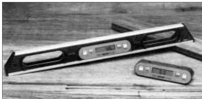
The triangular-shaped aluminum I-beam rail of the Pro SmartLevel is fitted with durable ABS panels and end caps, and the extra-large handholds can be grasped easily while wearing gloves. The electronic module mounts in the center handhold of the 24-inch rail and any handhold of the 48-inch and 78-inch rails.
