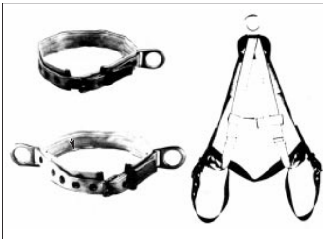
Figure 1. Safety belts come in two basic configurations. A one-ring belt (top left) is made to be worn with the ring centered on the back, so a worker will bend in a natural position when he comes to the end of a free fall. A two-ring belt with D-rings on each side (bottom left) is used only for positioning. If this belt is used to stop a free fall, the force can break a worker's back. A safety harness (right) offers the greatest protection because the shock is distributed across a worker's butt, back, and shoulders.
