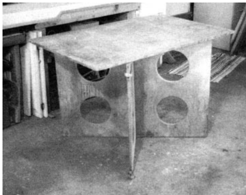
Figure 4. Lightweight, knockdown plywood supports make it easy to set up work stations at different heights (left). When not in use, the supports hang on the wall. At right is the pattern the author uses to make the supports.
