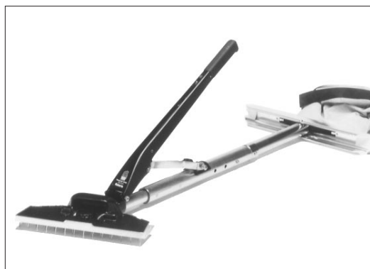
Figure 4. Since switching from jute backing to polypropylene, which is harder to stretch, many manufacturers will not warrant their carpet for rooms larger than 12x12 unless a power stretcher (left) is used during installation. A knee-kicker (right) is commonly used for small jobs, but it can cause knee problems with repeated use.
