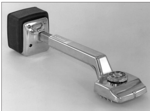
Figure 4. Since switching from jute backing to polypropylene, which is harder to stretch, many manufacturers will not warrant their carpet for rooms larger than 12x12 unless a power stretcher (left) is used during installation. A knee-kicker (right) is commonly used for small jobs, but it can cause knee problems with repeated use.
