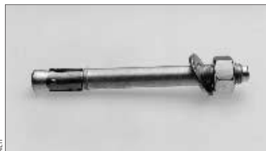
Figure 3. Wedge anchors. Often used in industrial construction, high-strength wedge anchors are also useful for attaching sills and ledgers. With soft substrates, however, a sleeve anchor or epoxy fastener is better.
