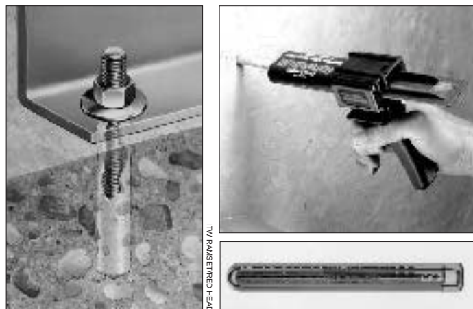
Figure 6. Chemical anchoring systems. Installed correctly, epoxy systems make the strongest anchors, and are ideal for joining foundations with rebar dowels. Unlike mechanical systems, they will work close to concrete edges (left), and can work in marginal substrates if reinforced with a wire-mesh sleeve. Modern dispenser systems (top right) have made the mixing process nearly foolproof. Capsule systems (bottom right) may be preferable if you're installing only a few anchors, but installation instructions must be closely followed to guarantee a good epoxy mix.
