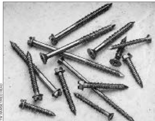
Figure 1. Concrete screws. Hardened-steel concrete screws cut their own threads into concrete or masonry. If the pilot hole is even slightly oversized, however, the screw is prone to strip out the hole.
