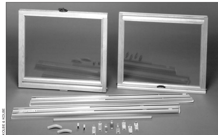
Figure 1. Sash-only replacement kits (left) include wood sash and vinyl jamb liners. Vinyl replacement units (right) typically have a vinyl frame around the jamb, making the replacement sash somewhat smaller.
