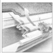
The WaterFall is installed without fasteners. A flat tab at the rear slips under the roof shingles, while the front snaps onto the gutter. It's available in white only, comes in 8-foot lengths, and costs about \$1.25 per linear foot. Contact Crane Plastics, 2141 Fairwood Ave., P.O. Box 1047, Columbus, OH 43216; 614/443-4891 or 800/726-7328.
