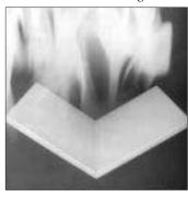
When I received my sample of Flamebreak, I took it outside and hit it with a blow torch. After several minutes, the only ill effect was a black surface patina. Designed as a covering for roof decks and firewalls, Flamebreak panels consist of a layer of APA-rated sheathing and a fiberglass-faced, silicone-treated gypsum backing. They're available in overall thicknesses of 5/8 inch or 3/4 inch, have a Class A flame spread rating, and have received model code compliance reports from BOCA and SBCCI.
