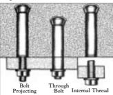
The Zykon concrete anchor is a European import developed for use in nuclear power plants. But don't let that throw you off. The anchor has been tested for safe working loads in cracks up to ½16 inch wide, making it useful for some residential applications in seismic areas.
