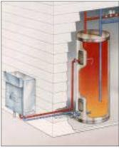
Want to lower your electric bills? If you live in a region with high rates and own an electric water heater, one option is to switch to gas. The Seahorse gas hot-water conversion system lets you convert from electricity to gas without buying a new tank. The self-contained Seahorse heater consists of a 28-inch-high, 18-inch-wide, and 12-inch-deep box that mounts on an outside wall. The "box" heats the water, while the old water heater serves as a storage tank.
