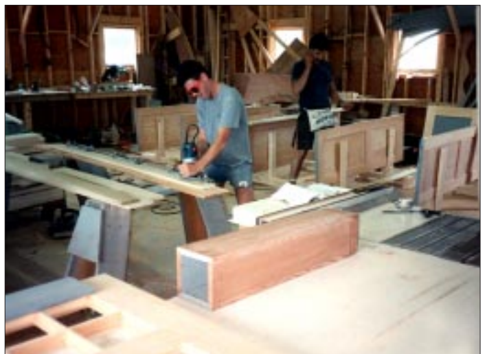
Figure 3. Prehanging doors. Even on high-end custom jobs, the author keeps costs in line by production-line preparation in the shop. Here, workers mortise a run of doors for a new house with a router and mortising jig.
