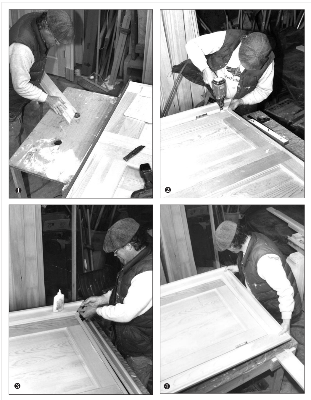
Figure 4. Precasing doors in the shop makes installation go quickly at the site. A table-mounted router with a slot cutter for biscuits (1) and a pneumatic finish nailer (2) speed the work. Two biscuits at each miter (3) produce tight-fitting, stable joints (4).
