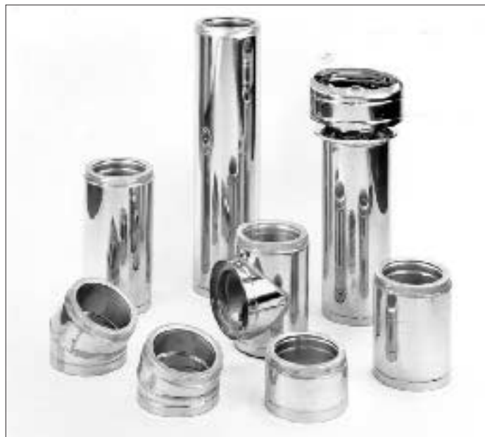
Figure 3. A Class A chimney is suitable for all fuel types, but it works better as a free-standing chimney than as a liner for an existing masonry chimney. The sections can be installed only in a straight chimney, and are extremely heavy, requiring a power winch and cable to lower them into place.
