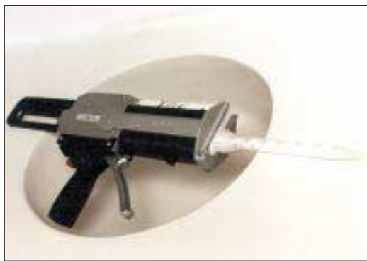
Figure 3. I'll be back. The author's crew called him Arnold whenever he picked up the futuristic-looking seaming compound applicator. The gun mixes the compound and catalyst in the correct proportions. The nozzle, which contains unused mixed portions, is disposable.
