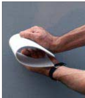
Figure 2. Much less brittle than plastic laminate, Nuvel will bend to tight radiuses without cracking.
