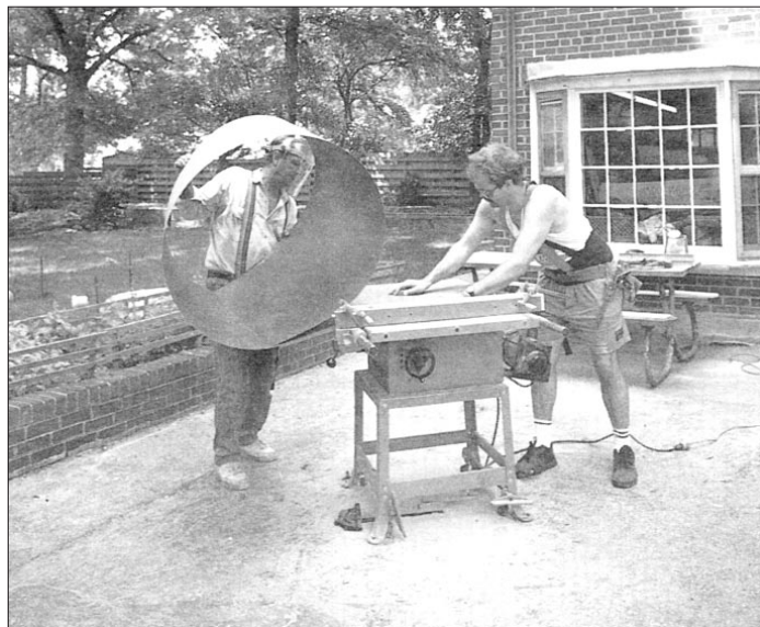
Figure 2. When ripping a full sheet of laminate on a table saw, unroll the sheet as you feed it into the blade and have a helper roll it up again on the outfeed side. A scrap of wood clamped to the saw fence eliminates any gap between the fence and the saw table.
