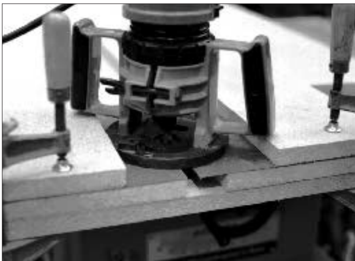
Figure 3. When making a laminate butt joint, cut both pieces at once using a simple particleboard jig. The base of the router rides against the top left piece of particleboard, which acts as a straightedge.
