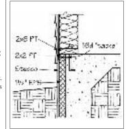
2x2 remains in the concrete, thanks to the nail heads from the tacking, and serves as a screed surface as well as a nailer for any door sills that might occur. Line the formwork below the 2x2 with 1½-inch EPS, and you're ready to pour. The nooks and crannies in the EPS bond mechanically and permanently with the concrete, the forms are a breeze to strip, and you can stucco over the EPS on the outside. Also, the EPS bridges any gaps in your formwork.
