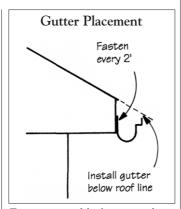
To prevent snow slides from tearing the gutter off, install gutters below the roof line, as shown.
