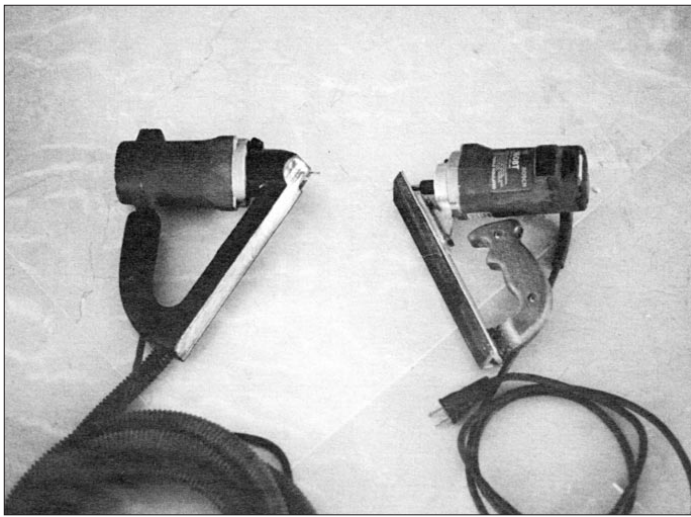
Figure 1. Both the RCT tool (left) and the Weatherhead tool (right) use a Bosch 1608T laminate trimmer motor mounted at a 45-degree angle to a V-shaped base. The base acts as its own fence in right angle corners, and the angle of the motor lets you rout into jamb corners.
