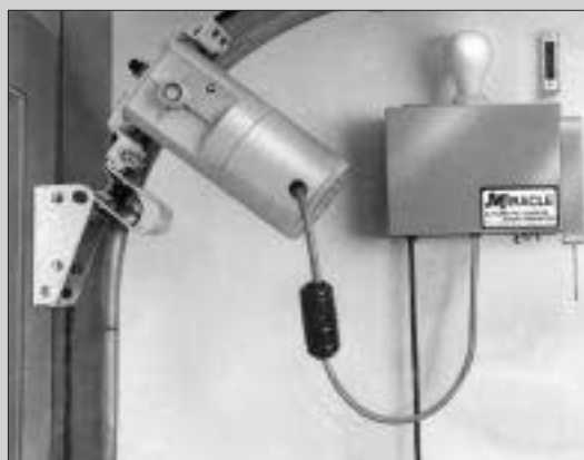
Figure B. The motor of the Miracle opener mounts to the door on a special replacement bracket that positions the drive wheel to ride on the garage door track. It requires no clearance beyond the path of the door to operate.
