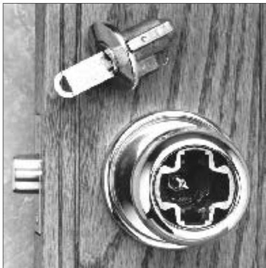
Figure 3. Kwikset's new Titan locksets feature a cylinder that can be removed for rekeying without removing the whole lockset. The cylinder is removed with a special key, as shown.
