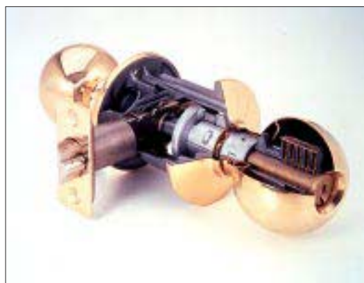
Figure 4. A bored, or tubular, latchset, like this Schlage F-series knob set, mounts in a round hole drilled in the face on the door rail. Note the deadlatch, a feature found on better latchsets, which prevents the springlatch from being forced back with a knife or credit card.
