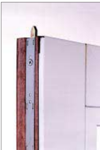
Figure 2. A cremone lock, shown here installed in a Pella door, has bolts that engage vertically into the floor and into the head jamb. This type of three-point lock offers excellent security and also helps prevent the door from warping, so the door always fits tight to the weatherstripping.
