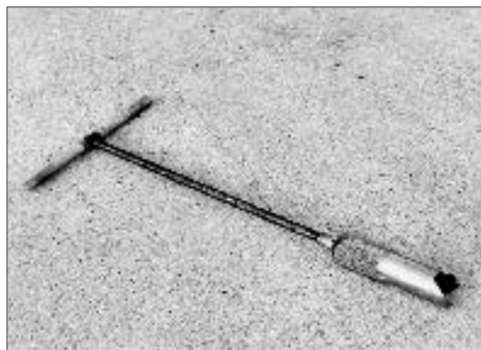
Figure 1. Use a hand auger for preliminary soil tests. There are two types: a pigtail auger, which has a spiral bit like a ship's auger, and a bucket auger, shown here. Both types are available with threaded extensions for probing deep below the surface.
