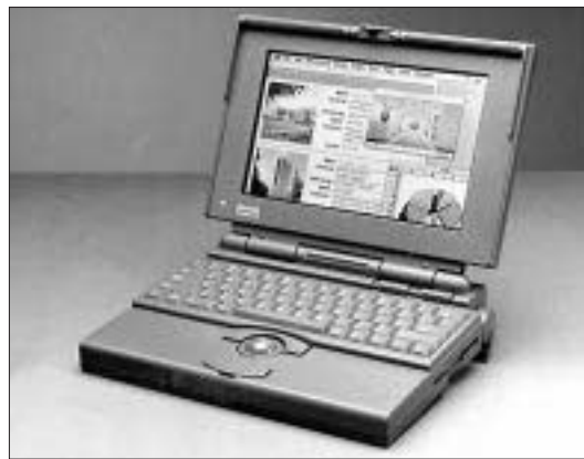
Apple's Powerbook 180 ($4,109 list with an 80-MB hard disk) weighs in at under seven pounds. The system comes with 4 MB of RAM and a built-in trackball.
