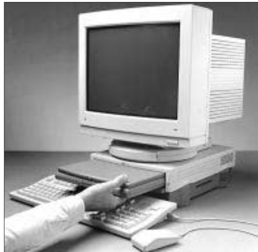
The Macintosh Duo System combines a lightweight portable computer with a stationary docking station, making it easy to switch between desktop and on-the-road computing.
