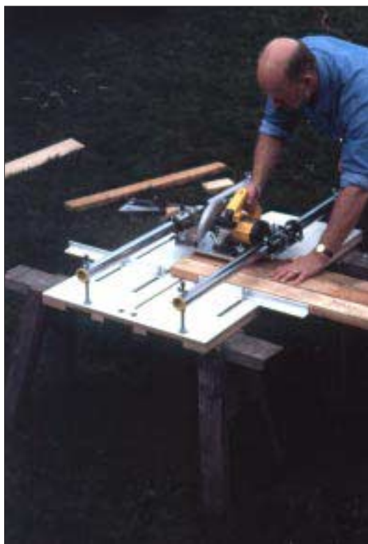
This Saw Trax cutting system works like a miniature panel saw with a cross-cutting capacity of 35 inches and a miter capacity of 21 inches. The saw carriage can be replaced to hold a router as well.
