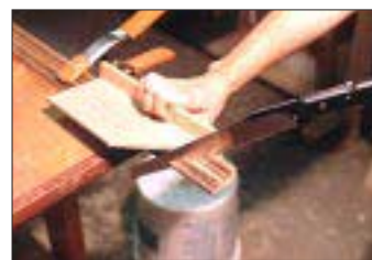
Figure 2. This simple jig works well to guide a Japanese handsaw when cutting a miter. The raised fence keeps the saw blade perpendicular to the face of the board, so the cut doesn't wander off at a slight bevel.
