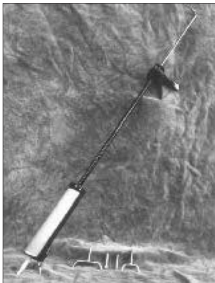
Figure A. The Goo Stick lets you spread adhesive on a set of joists while standing safely on a sheet of plywood. It includes a guide to keep the adhesive centered on the joist.
