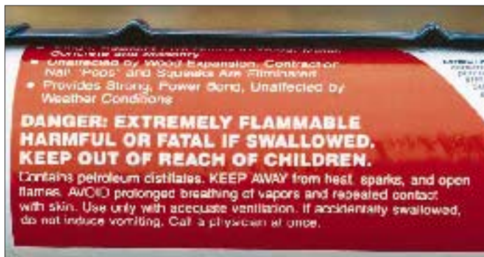
Figure 1. You can recognize solvent-based adhesives by the warning that they're flammable or a statement that they contain petroleum distillates.
