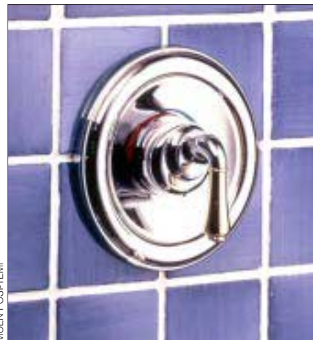
Figure 3. All pressure-balancing valves have single-handle controls. With one type, the handle rotates to adjust temperature and pulls out to adjust the volume (left). With cycling valves (right), there is no volume control; the lever turns the water on at full volume and rotates to adjust the mixed-water temperature.
