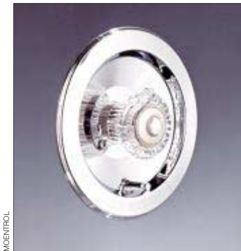
Figure 3. All pressure-balancing valves have single-handle controls. With one type, the handle rotates to adjust temperature and pulls out to adjust the volume (left). With cycling valves (right), there is no volume control; the lever turns the water on at full volume and rotates to adjust the mixed-water temperature.
