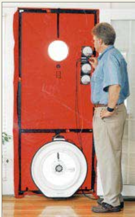
A blower door operator adjusts the fan speed to maintain a house depressurization of 50 Pascals.
