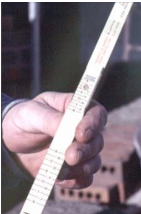
Figure 4. The author uses an oversize ruler, marked with letters rather than numbers, to gain or lose height incrementally. The higher the letter used, the greater the height of each course. By adjusting course height, the author minimizes cutting of bricks below window sills and soffits or above headers.
