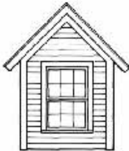
Figure 1. Small doghouse dormers look best if they are not too wide (left) nor too tall (center). The author tries to match the pitch of the main roof, and keeps dormer overhangs in proportion to the dormer (right).
