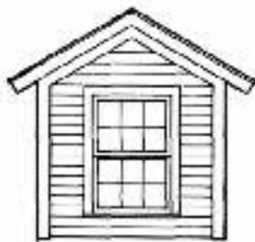
Figure 1. Small doghouse dormers look best if they are not too wide (left) nor too tall (center). The author tries to match the pitch of the main roof, and keeps dormer overhangs in proportion to the dormer (right).
