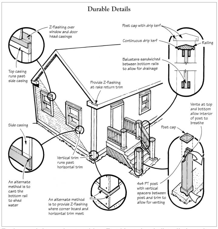
The author uses several techniques to make exterior trim shed water. These include canting the top edge of horizontal boards, routing drip grooves on the underside of railings, and avoiding exposed end grain wherever possible.
