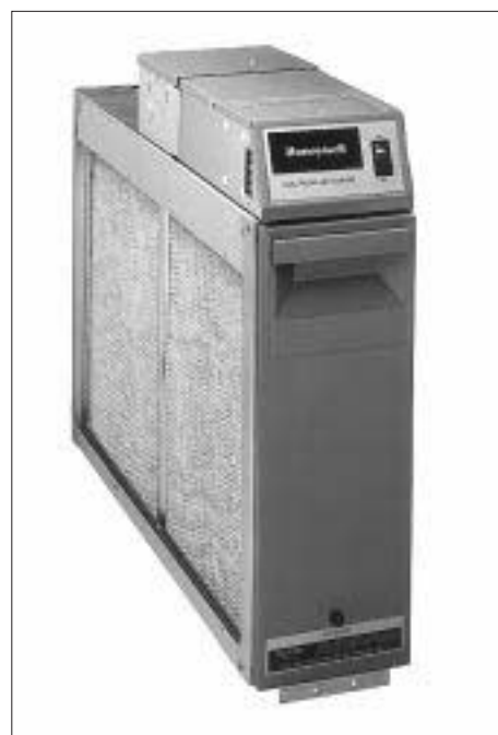
Figure 3. An electronic air cleaner mounts on the return side of the air handler. Dust particles passing through the unit are energized by a set of electrically charged plates and wires, then captured by a set of oppositely charged collector plates.
