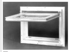
The Acrolin eis a welded-frame custom vinyl window with hardware that lets you convert it from an awning to a hopper. Designed for use in a full basement, it includes single-glazed or 5/8-inch thermopane glass. When used as an awning, two sets of stops let you open the window to 45 or 90 degrees (but not to any other settings). The hopper relies on a chain to hold the sash open at 45 degrees.
