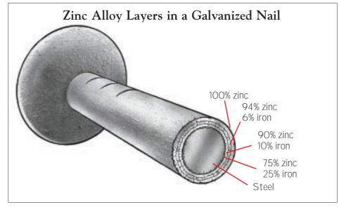
According to the American Galvanizers' Association in Aurora, Colo., hot-dip galvanizing creates a series of protective alloy layers around a steel nail. The outer layer is 100% zinc, while inner layers contain progressively less zinc and more steel. If the zinc and alloy layers are scratched and some steel is exposed, zinc in the outer layers will corrode before the steel does, preventing rust formation.
