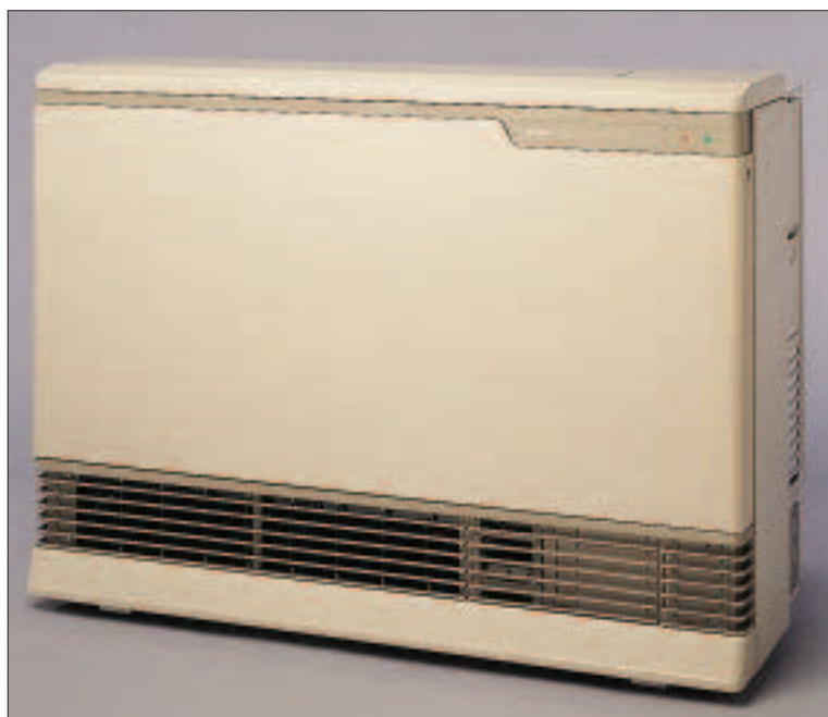
Figure 7. The Rinnai wall-mounted gas space heater vents to the outside through a short concentric pipe. The inner pipe carries exhaust, while the outer pipe brings fresh air to the burner. With electronic ignition and power venting, these heaters have AFUEs of more than 80%.
