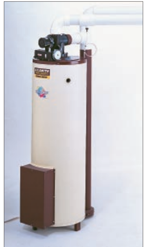
Figure 4. Some gas water heaters, such as this State model 850 (left), use a concentric pipe (also called “coaxial” or “double channel” pipe) for both venting and combustion air. Since this type of unit relies on natural venting to move exhaust out of the house, it must be installed close to the outside wall. Water heaters with integral power venters, such as the A.O. Smith Sealed-Shot (right), may be installed as far as 40 feet from an outside wall.
