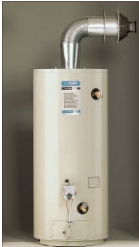
Figure 4. Some gas water heaters, such as this State model 850 (left), use a concentric pipe (also called “coaxial” or “double channel” pipe) for both venting and combustion air. Since this type of unit relies on natural venting to move exhaust out of the house, it must be installed close to the outside wall. Water heaters with integral power venters, such as the A.O. Smith Sealed-Shot (right), may be installed as far as 40 feet from an outside wall.
