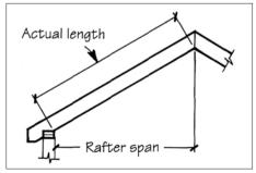
Use the horizontal projection of a rafter, not its actual length, when figuring rafter span.
