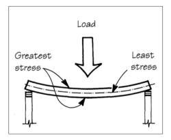
As a structural member bends, the fibers along its upper and lower edges are highly stressed, while those near the center are not stressed at all. Fb ("extreme fiber stress in bending") is a measure of the stress that can be placed on these outermost (or "extreme") fibers; the higher the Fb, the stronger the wood.
