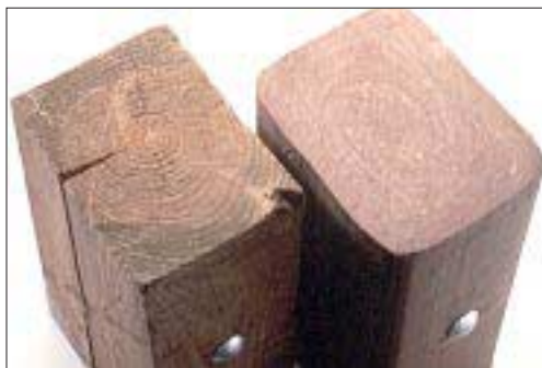
Unlike wood, Trex (at right) is completely uniform — no checks or knots.
