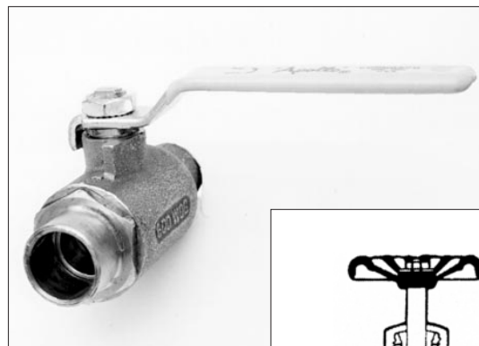
Figure 1. The author uses only full-flow valves, like this Apollo ball valve (above), in water supply lines. Globe valves (right) may be cheaper, but they restrict water flow.
