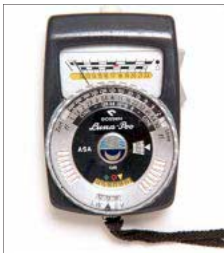
Figure 2. An incident light meter directly measures the intensity of the light source. By taking several readings, you can adjust the lighting so all important details are well lit.
