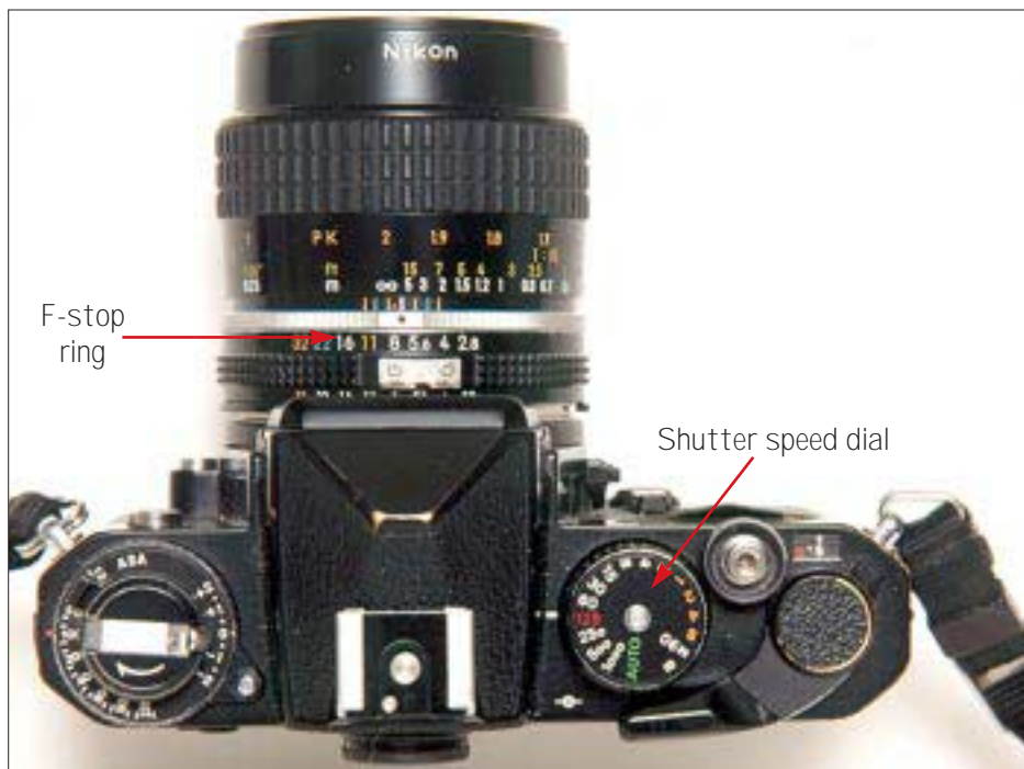
Figure 3. The shutter speed dial on the top right of this camera is set to 1/125 second — the amount of time the film is exposed to light. The f-stop ring on the lens is set to 8. Higher f-stop numbers close the aperture; lower numbers open the aperture.
