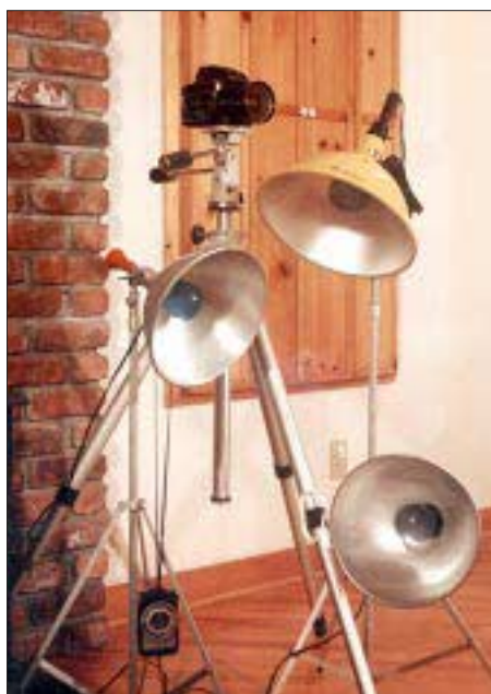
Figure 1. The author’s equipment includes inexpensive photoflood sockets with 10- and 12-inch-diameter reflectors, 250-watt and 500-watt color-balanced bulbs, a sturdy tripod, a medium-format camera, and an incident light meter.
