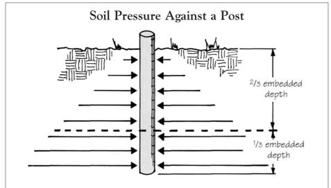
**Figure 1.** The pressure of the earth against an embedded post increases as the post goes deeper. According to the Coulomb theory, the pressure against the bottom third of the post equals the pressure against the top two-thirds.
