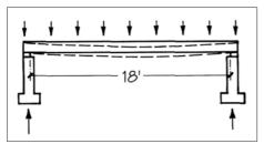
Watch out for floor spans over 18 feet — these push the limits of dimensional lumber for strength and stiffness.
