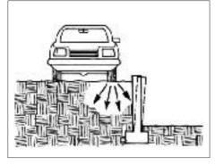
A car parked near a retaining wall increases the soil's lateral pressure against the wall.
