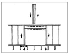
Though it may solve an architectural design problem, a point load on a header can create structural problems in the surrounding framing.
