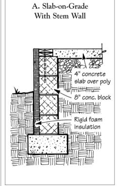
This slab-on-grade foundation is a poor choice in areas where termites are a problem. Termites can slip through the foundation/slab joint, inside the hollow concrete blocks, or between the insulation and foundation.
