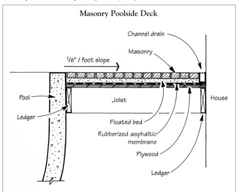
Masonry, floated over a membrane-protected wooden structure, is a durable choice for a poolside deck. Slope the surface away from the pool and install a channel drain around the perimeter of the deck.
