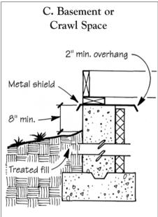
A monolithic slab (top) or a cast concrete wall (above) presents fewer entry routes than a slab resting on a stem wall. It's important to leave at least 8 inches of the foundation exposed above grade. Although some insulation value is lost, this allows an exterminator to inspect for the presence of termites.
